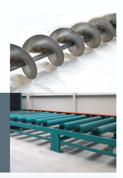
The screw conveyor is designed with a spiral made of structural steel and transports the steel granules. There is a Hardox-500 steel plate on top to prevent large parts from falling into the screw conveyor. And this steel plate also protects the screw conveyor from rapid wear.
